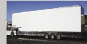
2004 RENEGADE STACKER TRAILER 3 CAR WITH CABINETS AND LIFT TRIPLE AXLE, GOOSE NECK
